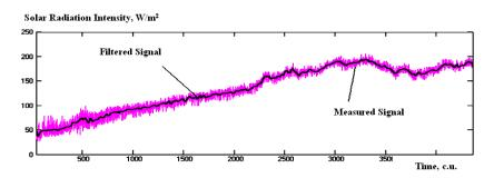
Fig. 4. Imposition of the incoming signal and the filtered time series of solar radiation intensity
