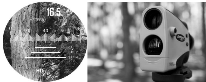
Fig. 1. TruPulse 360B with built-in scale for remote measurement of stem diameters
