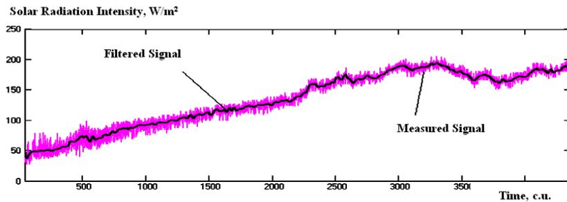
**Fig. 4. Imposition of the incoming signal and the filtered time series of solar radiation intensity**
