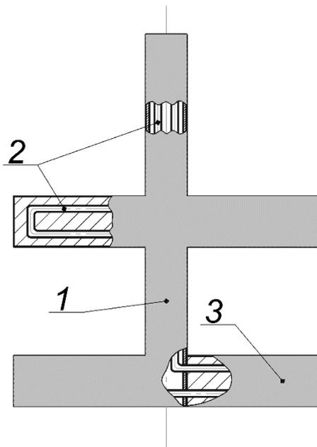
**Fig. 1. Combined system for mixing and electric heating: 1 – shaft; 2 – electric heating cable; 3 - paddle**
