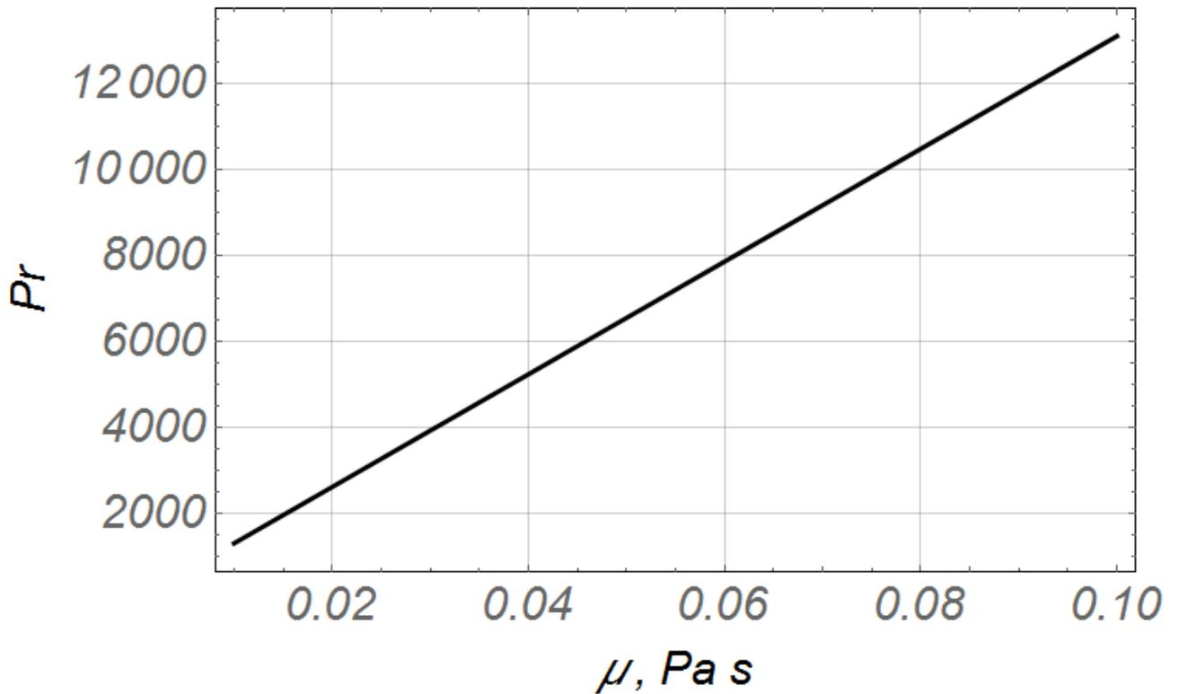
**Fig. 5. Dependence of the change in the Prandtl similarity criterion on the change in the dynamic viscosity of the substrate**
