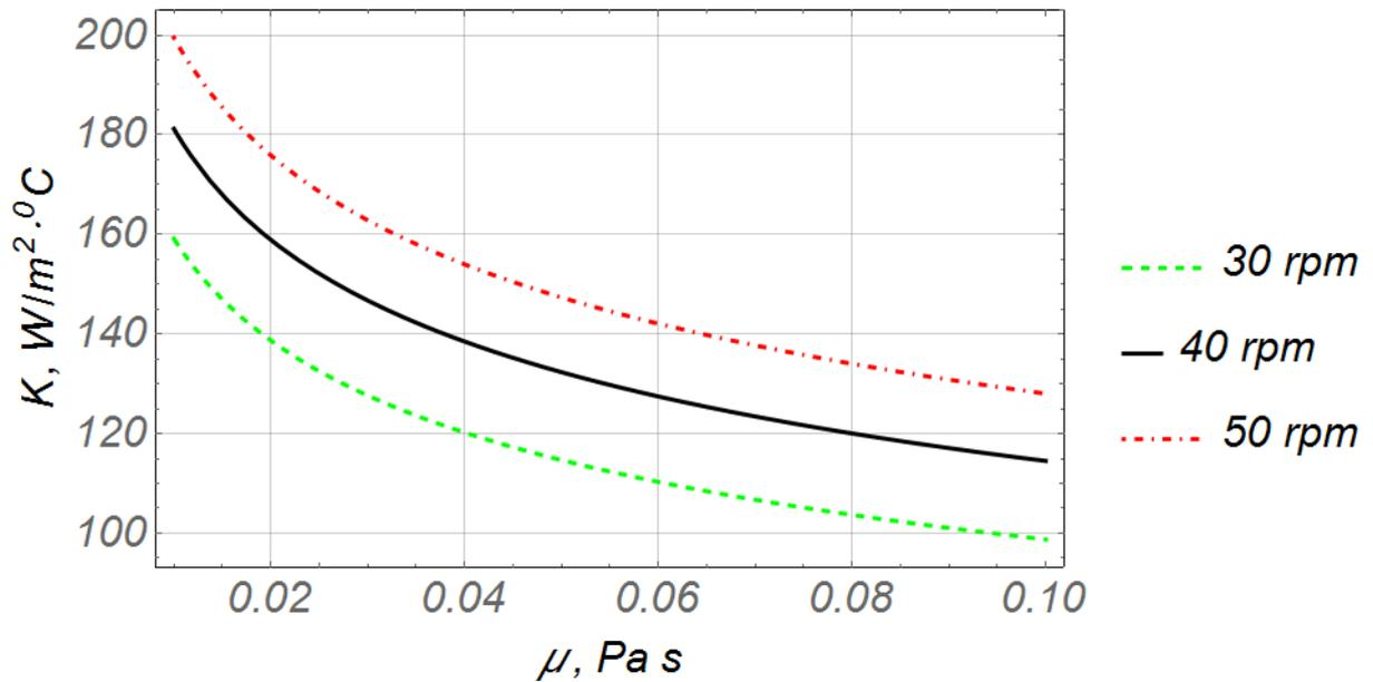
**Fig. 4. Dependencies of the change in the heat transfer coefficient ( $k$ ) depending on the change in the dynamic viscosity of the substrate and the frequency of rotation of the working body of the mixing device**
