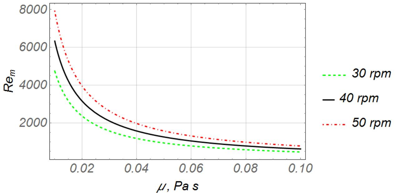
**Fig. 2. Dependencies of the change in the Reynolds criterion depending on the change in the dynamic viscosity of the substrate and the frequency of rotation of the working body of the mixing device**
