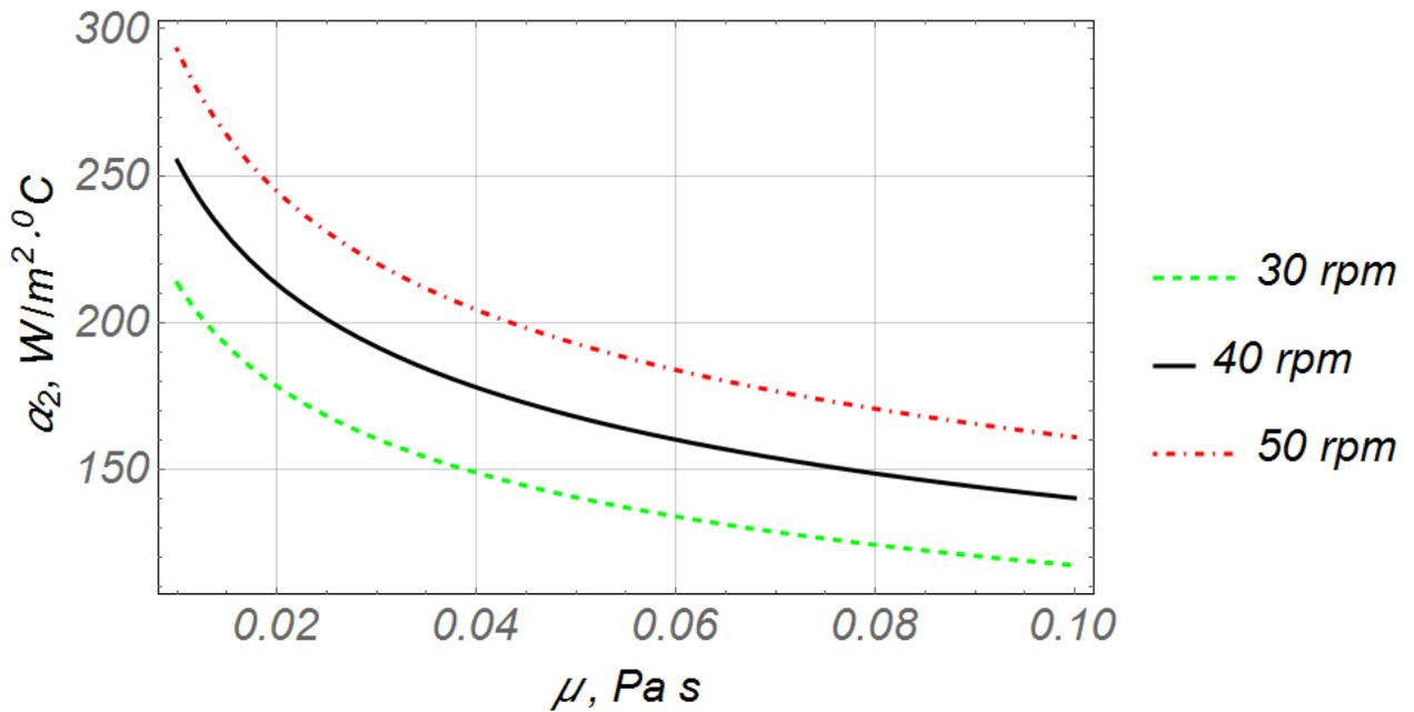
**Fig. 3. Dependencies of the change in the heat transfer coefficient ( $\alpha_2$ ) depending on the change in the dynamic viscosity of the substrate and the frequency of rotation of the working body of the mixing device**
