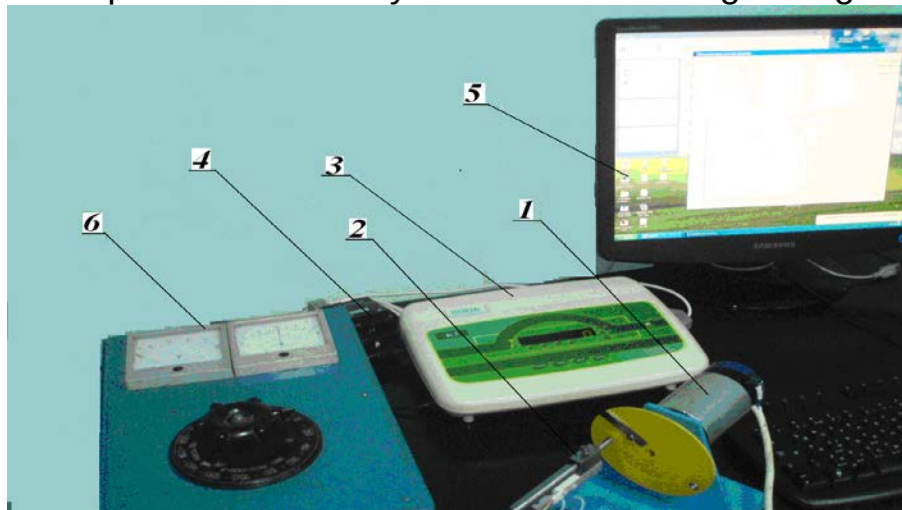
Fig. 2. Measuring system for determination of dynamic cutting forces feed grains: 1 - a device for cutting; 2 - strain gauge; 3 - Weighing terminal; 4 - analog-to-digital converter; 5 - PC; 6 - power supply.
