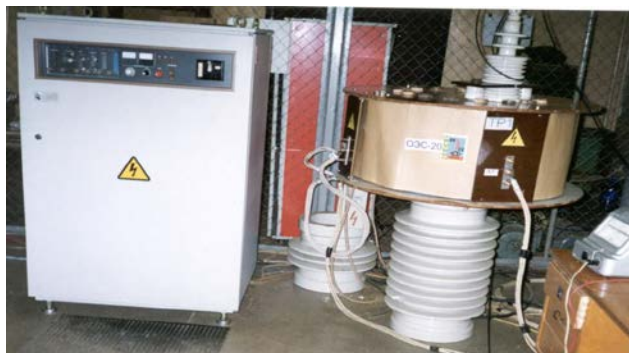
Fig. 7. 20 kW, 1 kHz resonant electric power transmission system.
