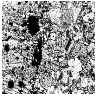
Picture 4. Microstructure contact with the material CPM-0.2 after 100 000 switching
