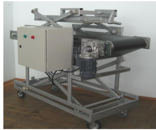
Fig. 6. Electrotechnological complex magnetic processing of agricultural products
