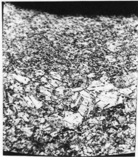
Fig. 5 Microstructure anode contact material CPM-0.2 1h105 after switching.
