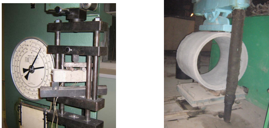
Fig. 1. Test fiber concrete beams reinforced fiber and microcrystalline basalt fiber concrete wall rings Ø 1000 mm.
