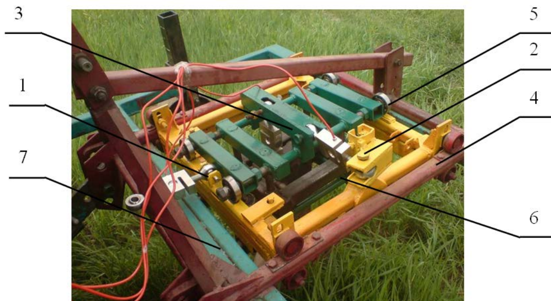
Fig. 1. Experimental setup: 1, 2, 3 - sensors for measuring respectively the longitudinal, lateral and vertical component of the resultant force of resistance; 4, 5, 6, 7 - frames, which see under longitudinal, lateral, vertical components of the resistance and the resulting frame for attachment of the assembly to the tractor [7].
