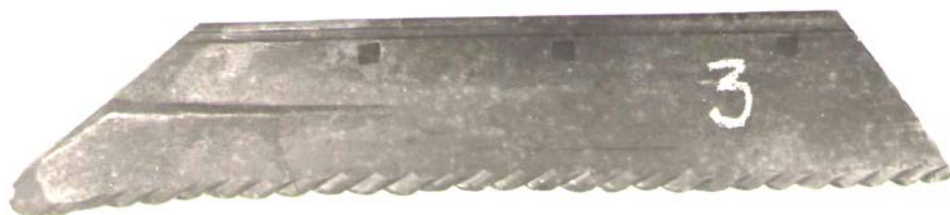
Fig. 8. ploughshare plow operating time after 49 ha.
