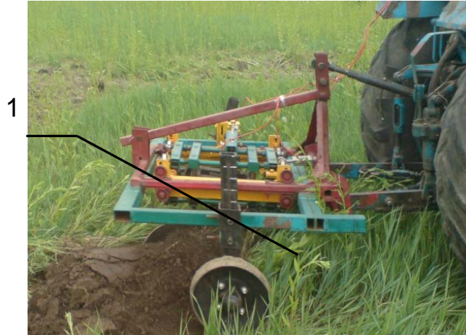
PIP. 5. Plowing plow body of experimental shelf: 1 - supporting wheels
