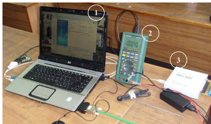
Fig. 11. Equipment collect data from the experimental setup: 1) PC; 2) Multimeter; 3) Module ADA.
