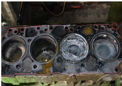
Fig. 5. Application of purified biogas as the fuel – no destruction and corrosion effects are visible
