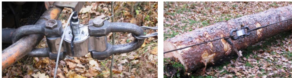
Fig. 4. DCHV-01 sensor for contactless control of the rotation frequency detail components and mechanisms: and - a general view; b - placing the sensor on the shaft of the drum.
