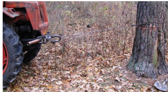
Fig. 5. measure force sensor K-20-R: And - a general view; b - placing the sensor on the towing rope; in - prozmeshchennya sensor rope-stretching.
