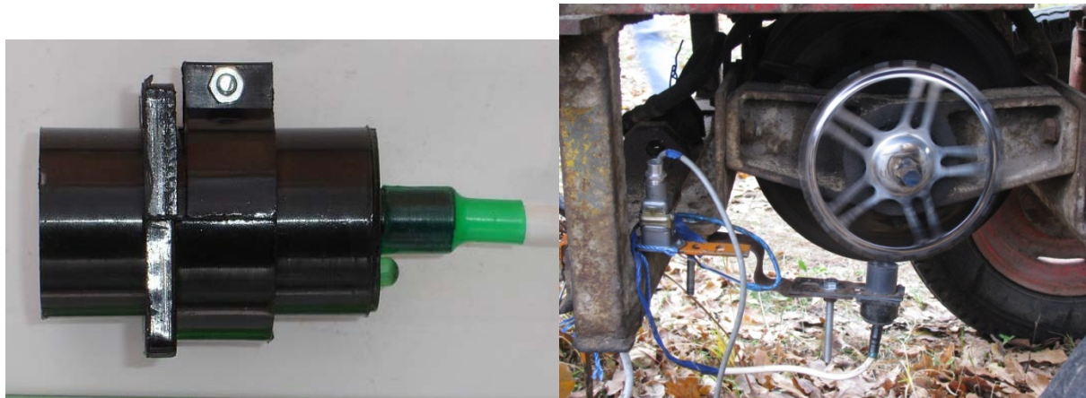
Fig. 4. DCHV-01 sensor for contactless control of the rotation frequency detail components and mechanisms: and - a general view; b - placing the sensor on the shaft of the drum.
