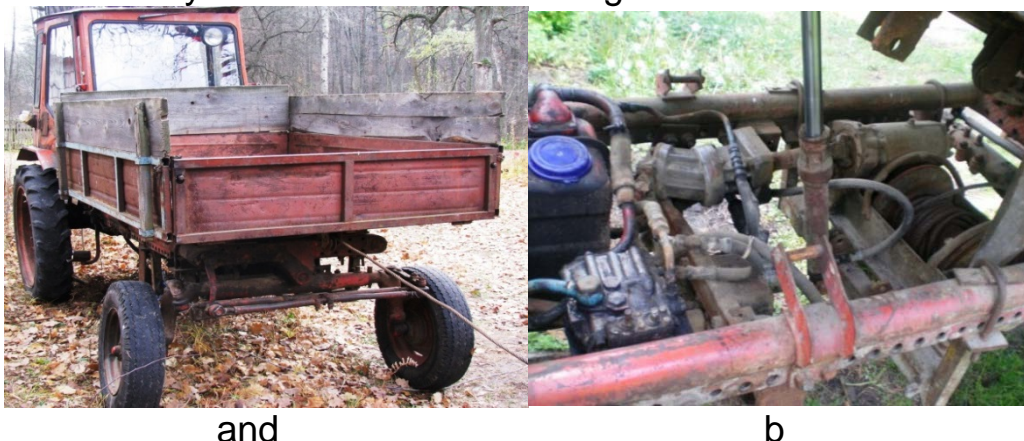
Fig. 1. Full-scale model of forest machine odnobarabannoyu winch: and - a general view; b - winch drive layout.
