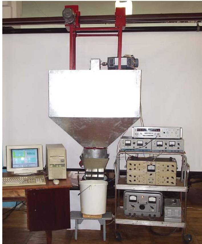
Fig. 2. General view of the stand for the study of individual workers distributor dosing feed.
