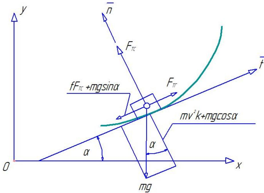
Fig. 2. Expansion of the forces to start normal  $\bar{n}$  and tangent  $\bar{t}$  curve.
