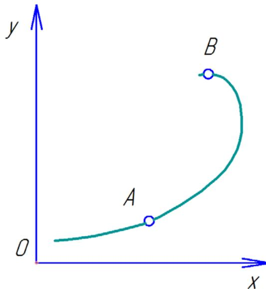
Fig. 3. The curve that provides constant pressure at a constant speed of particles:  $a_{tc} = 1.2$ ;  $v = 0,2$  m / s.
