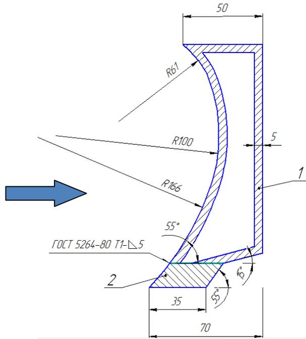
Fig. 4. Designed scraper scraper installation.
