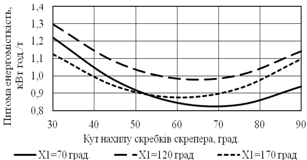
Fig. 6. Dependence of specific energy intensity improved scraper installation on the angle scraper scrapers.
