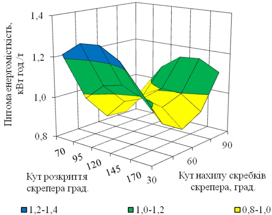
Fig. 7. Dependence of specific energy intensity improved by installing angle scraper opening and the angle of inclination scrapers scraper.
