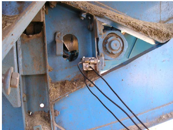
Fig. 1. Measuring vibration threaded connection technology.
