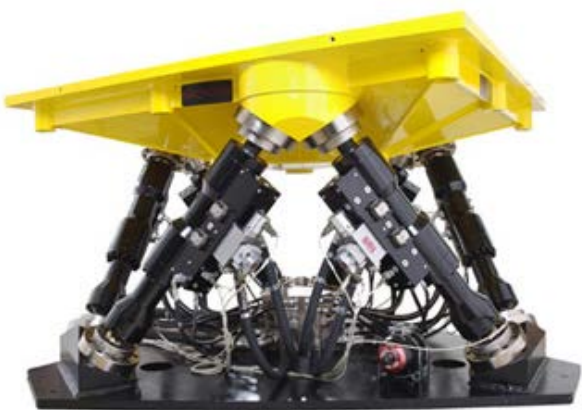
Fig. 1. Vibration setting MOOG (USA): frequency range - low, medium, high; number of degrees of freedom - 6; Drive - hydraulic servo; computer system management mode oscillation.
