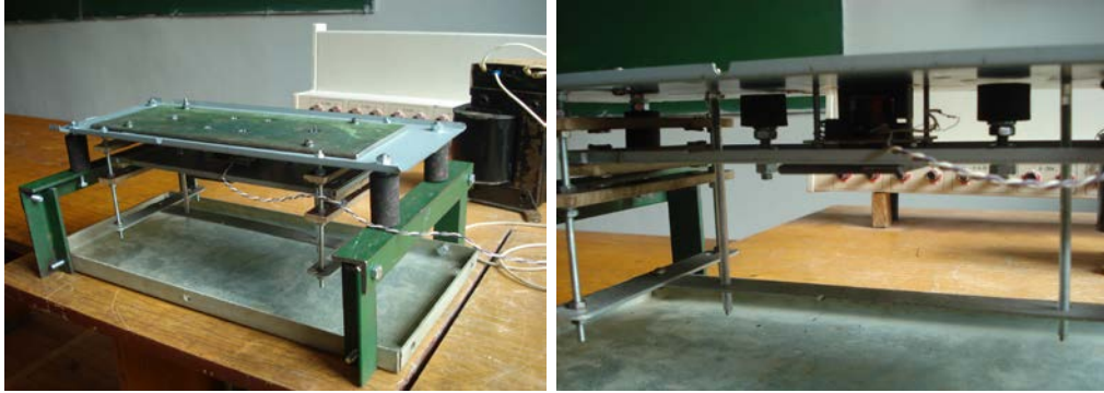
Fig. 10. Laboratory dvomasova electromagnetic shock-vibration installation of redesigned suspension drummer.
