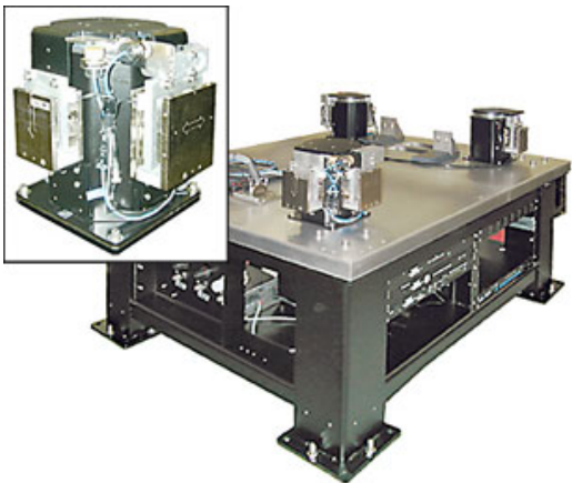
Fig. 2. Vibration setting TMC (USA): frequency range - > 100 Hz; number of degrees of freedom - 6; Drive - electromagnetic exciters; digital control system.
