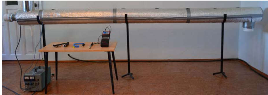
Fig. 1. Technological scheme (s) and general view (b) experimental stand 1 - two-pipe module; 2 - small cap; 3 - large cap; 4 - trumpet; 5 - a fan controller performance.
