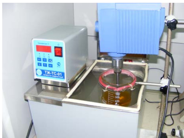
Fig. 3. The laboratory setting to determine the influence of parameters on the mixer alkalinity biodiesel.
