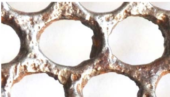
Fig. 3. The uneven surface of the sieve as a result of blows hard patches.
