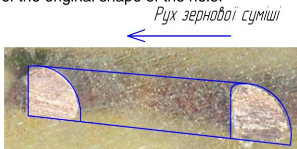
Fig. 1. Cross-section of worn hole sieve crusher.
