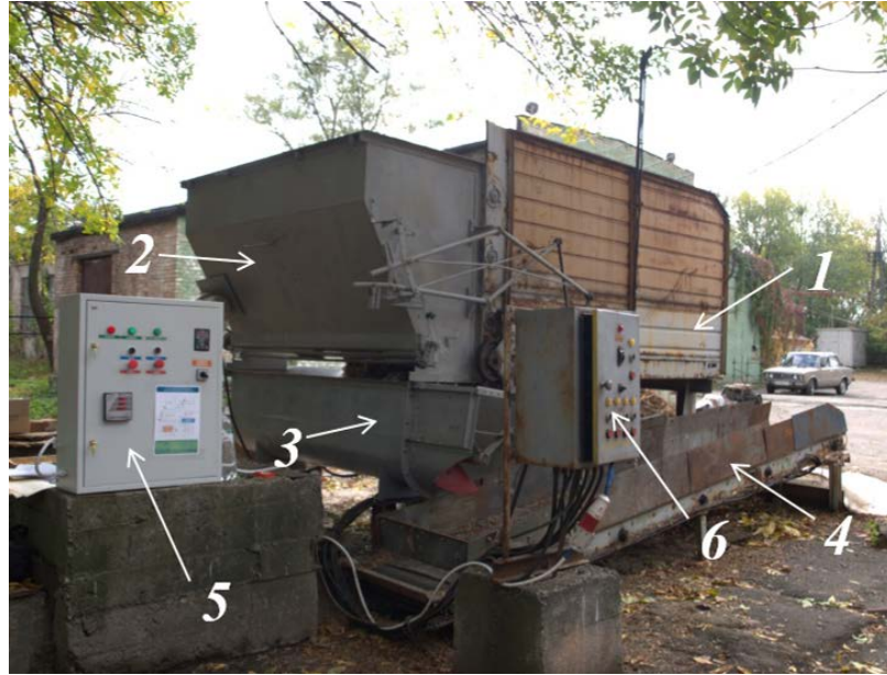
Fig. 1. The experimental pilot plant at the mixer-feeder stream type 1 - hopper feed dispenser stem; 2 - tank dispenser kontskormiv; 3 - vane mixer; 4 - conveyor belt; 5 - motor control unit and measure power consumption; 6 - flap control motors.
