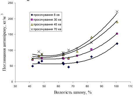
Fig. 1. Dependence of the absorption of moisture retardant veneer.
