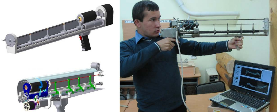
Fig. 1. Model of mobile devices for measurement Resistance sverlenyyu (diagnosis STATUS timber) patenty RF №95128, №2448811 (left); laboratornaya Experimental setup for diagnosis STATUS timber sverlenyem (right).
