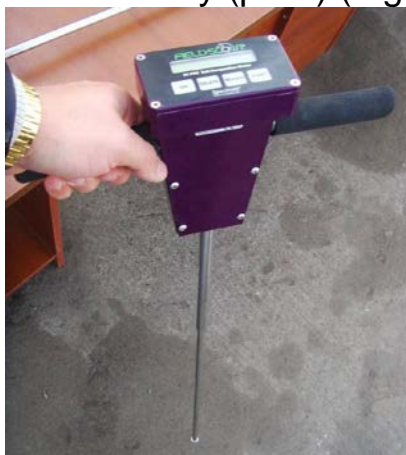
Fig. 8. penetrometer to determine the properties of the soil.
