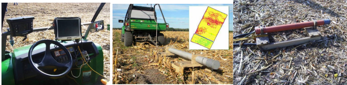
Fig. 6. A device for determining the conductive properties of the soil by touch.
