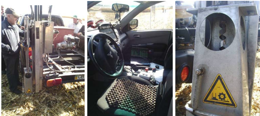
Fig. 3. Automatic auger sampling of soil samples.
