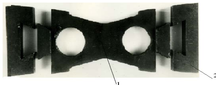
Fig. 1. The design of hammer crusher DB-5 (DCM-5): 1 - the basis hammer, steel, Art. 3; 2 - operating (variable) part of the wear-resistant material.
