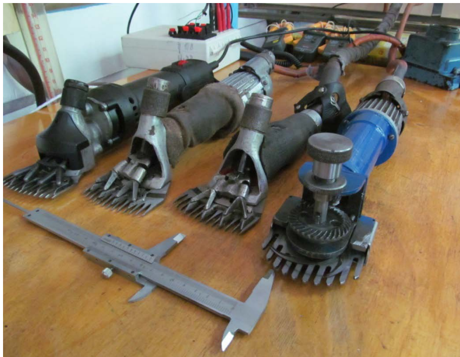
Fig. 1. Investigated stryhalni machines: from right to left: N1J-GM01-76, ISU-200 MSO77V stryhalna machine and rotary type.
