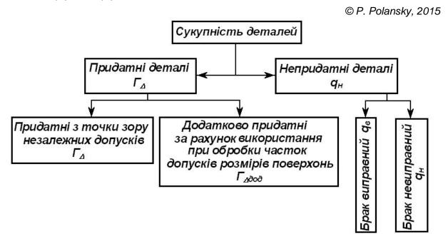
Fig. 1. Classification by Category parts life with dependent tolerances.
