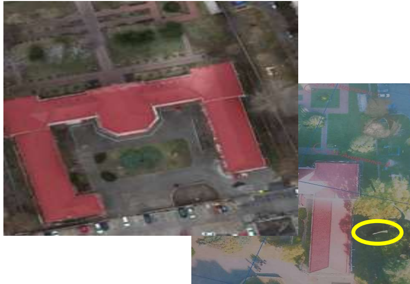
Fig. 3. "Breaks" of the orthophotomap image when using different algorithms for its construction
