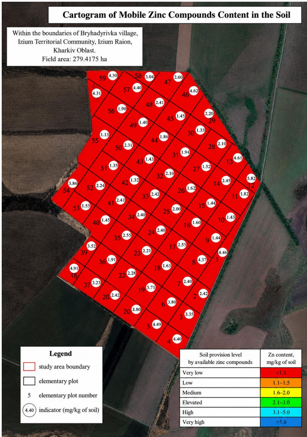
Figure 8. Cartogram of the Spatial Distribution of Mobile Zinc Compounds Content in the Soils of the Investigated Land Plot
