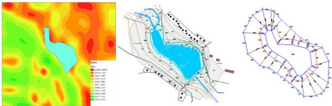
Picture 3. Cartogram of slope steepness, plan-scheme and layout drawing of the established boundaries water protective zone and the coastal protective stripe around the pond in Gremyache village, Rivne region
