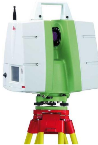
Figure 3. Leica Total ScanStation C10
