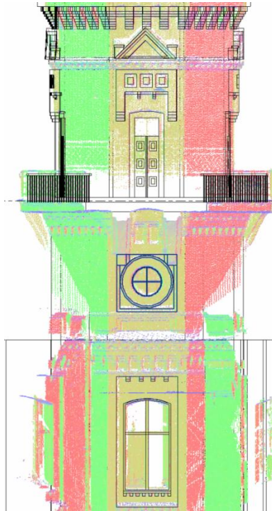
Figure 7. High-precision 2D drawing based on a BIM model
