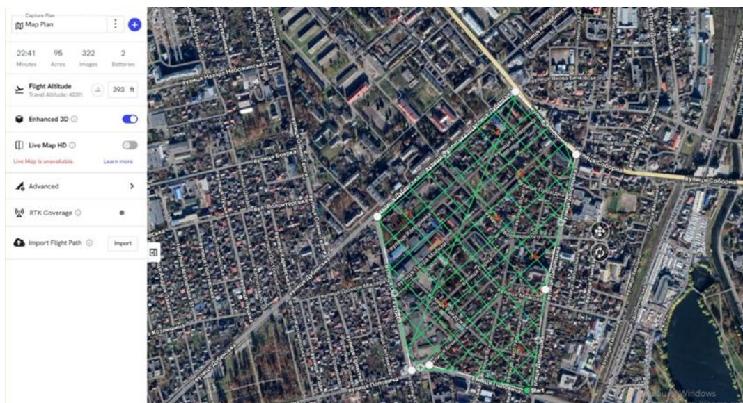
Fig. 4. Planned aerial survey route using the DroneDeploy Flight App.
